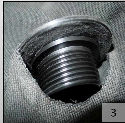
Insert Scubapro repair valve
