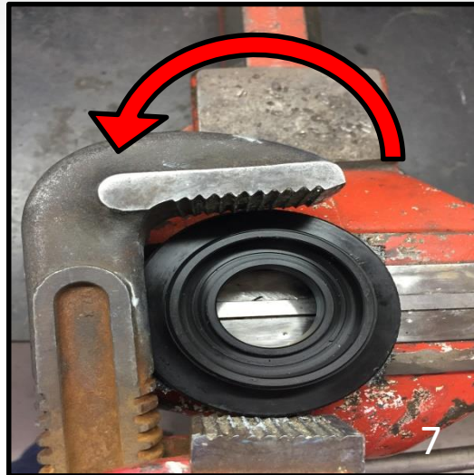
18" Pipe Wrench Gripping On The Lock Ring.
