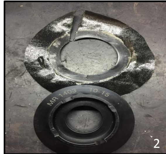
Valve After Removing Old Fabric.
