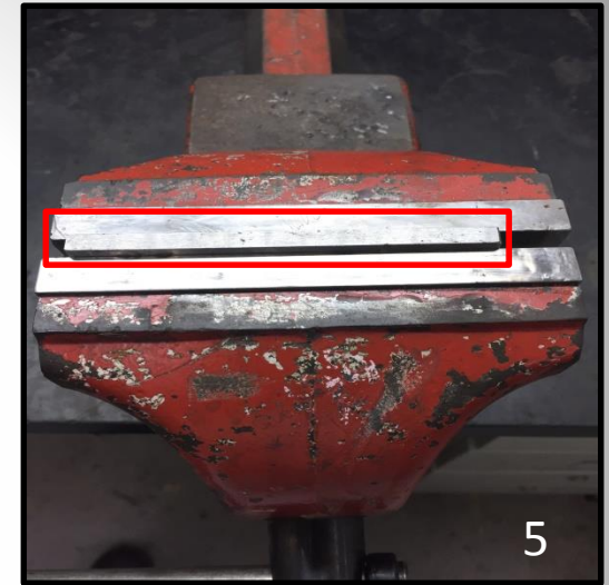
Clamp 6mm Square Block Onto A Bench Vice
